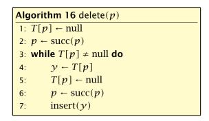
$\boldsymbol{p}$  is the index into the table-cell that contains the object to be deleted.
