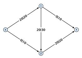
From the graph G = (V, E, c) and the current flow f we construct an auxiliary graph  $G_f = (V, E_f, c_f)$  (the residual graph):
