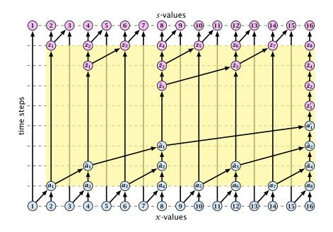
The algorithm uses work  $\mathcal{O}(n)$  and time  $\mathcal{O}(\log n)$  for solving Prefix Sum on an EREW-PRAM with n processors.
