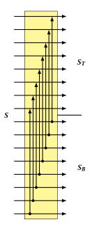
If we feed a bitonic 0-1 sequence S into the network on the right we obtain two bitonic sequences  $S_T$  and  $S_B$  s.t.
