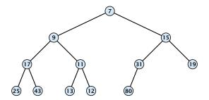
Nearly complete binary tree; only the last level is not full, and this one is filled from left to right.
